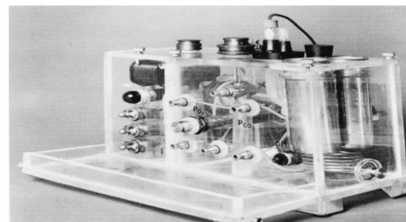
Fig. 2. First three-function blood gas apparatus (pH, partial pressure of carbon dioxide [Pco 2 ], and partial pressure of oxygen [Po 2 ] electrodes) built by Severinghaus and Bradley (1959).
